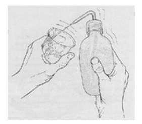
Add the rinse water to the mixture in **beaker #1**. Rinse **beaker #2** again with distilled water and this time discard the rinse water. The clean beaker will be used again in step i.
