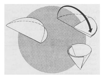
Fit it into a funnel and moisten the paper with some distilled water from a wash bottle to make it stick to the glass. Set up the funnel for filtering as shown in Fig. 8-5.
